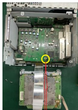
1).After disassembling the panel, cover and the screws of the original engine, install the copper column in the position specified in the figure.
