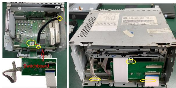
2).Insert the 50PIN and 12PIN line on the switching board with the original headunit, fix the switching board with the screws removed from the original headunit, and then insert the LVDS line and pay attention to the outlet position. The movement and upper cover are then installed, as shown above.
