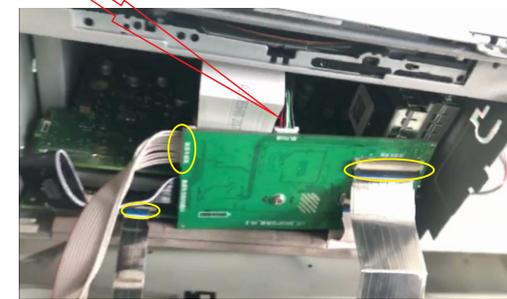
3).Insert the three lines of the original headunit's panel (50PIN FPC/12PIN/SD card cable).Then restore the panel of the headunit.
